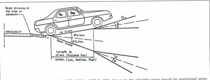
\* Shoulder slope usually varies from ½"/ft. (4%) to 3/4" ft. (6%). However, the shoulder slope should be maintained when constructing the driveway,
