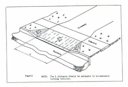
(B) If the driveway grade would exceed 8.0%, depress the outer edge of the sidewalk and maintain a maximum sidewalk cross slope of 6.0%. This will enable the driveway slope to stay within the 8.0% slope limit. See Figure 3.
